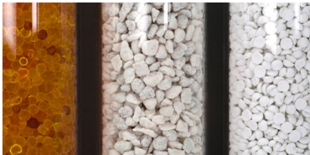
Silica gel, humidifier granules and soda lime for H 2 O and CO 2 control
