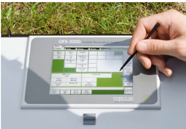
Color screen with touch panel, well readable in sunlight
