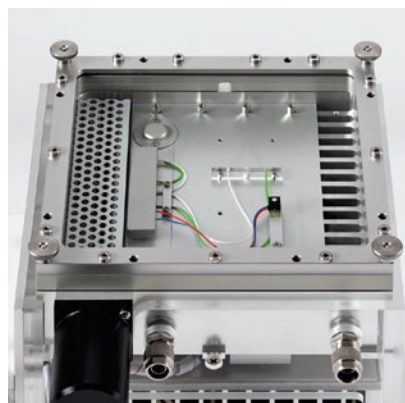
Gas-Exchange Chamber 3010-GWK1, top view showing sample area and sensors
