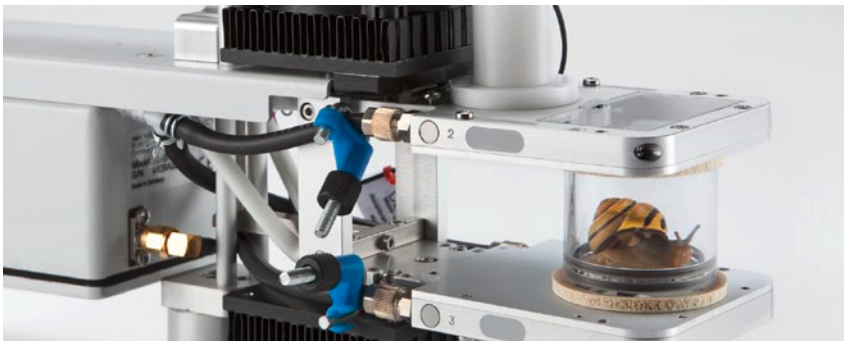
Lichens/Mosses Cuvette 3010-V32 here used to measure gas exchange of a small animal
