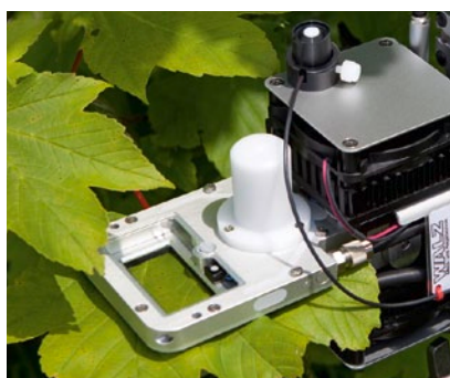
Standard Measuring Head 3010-S with Light Source 3040-L and darkening plate connected
