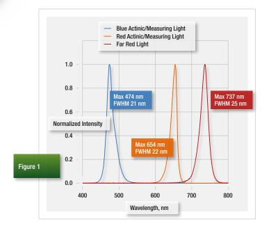
Figure 1: Typical LED emission spectra normalized to their maxima. The blue curve corresponds to the spectrum of the blue LED of the MINI-PAM-II/B, the orange curve represents the red LED in the MINI-PAM-II/R. Both MINI-PAM-I versions possess a far red LED which emits maximally above 700 nm (rightmost curve). Max, peak wavelength in nm. FWHM, full width at half maximum in nm.
