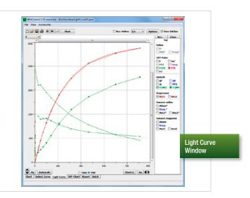
Light Curve Window: Fluorescence data are plotted against PAR. Red points represent ETR data to which the light curve model "REG1" was fitted by WinControl-3 (dark red curve). Using green color, the panel displays three types of photosystem II quantum yields: the yield for photochemistry (Y(II), steeply declining), for uncontrolled heat dissipation (Y(NO), shallowly declining), and the yield for controlled heat dissipation (Y(NPQ), rising).
