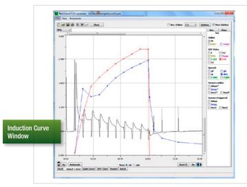
Induction Curve Window: The window displays continuous PAM fluorescence (Ft) as black line. The non-photochemical quenching parameter, NPQ, is drawn in blue and electron transport rates (ETR) are shown in red.
