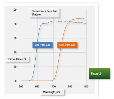
Figure 2: Transmittance spectra of detection filters in the MINI-PAM-II-B (blue line) and MINI-PAM-II/R (orange line).
